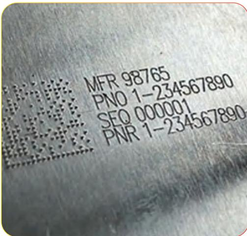
HS-DE series plate marking machine is compact and portable, no need connect air compressor to work, HS-DE04 your side just plug and play, HS-DE05 need connect computer to use, software is all windows support, the machine often engraves on follow parts,
